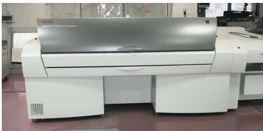
CtP Kodak Magnus VLF Quantum Platesetter 5183
